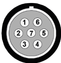
Figure 1: Pin assignment input (socket view, device) Use this plug: LEMO FGG.1B.307
