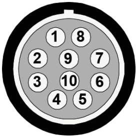
Figure 2: Pin assignment system link (socket view, device) Use this plug: LEMO FGG.2B.310...
